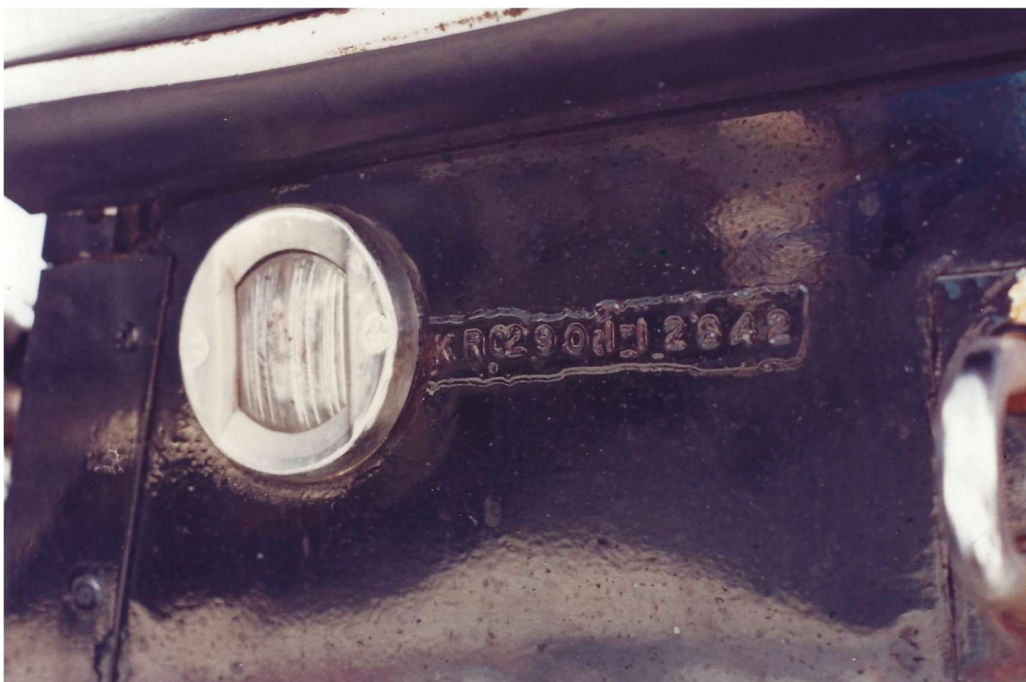
Altered Hull Identification Number
